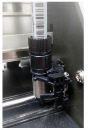
Next, take the pen out of the height gauge and place it into the holder on the right of the machine. Gently pull the spring loaded foot toward you and slide the collet into the holder. Do this while the machine is off. Ensure that the pen is located EXACTLY as in the image to the left, with the top channel fitting into the semicircular holder and the spring clip grabbing onto the lower channel.
